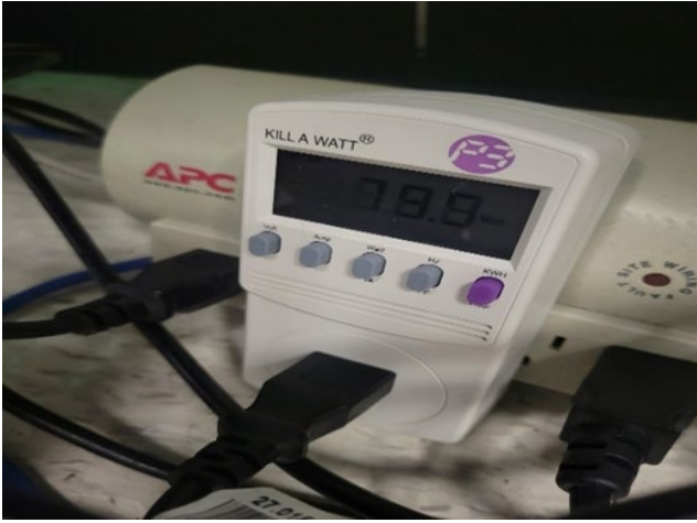
Fig. 11. P4400 p3 Kill-A-Watt meter for measuring power usage of each model during training.
